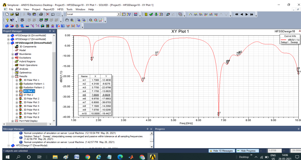
Figure 15: Return Loss Plot of the Slotted Antenna with Elliptical D.G.S.
